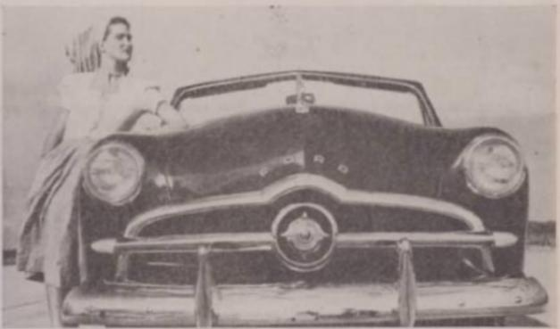
The smooth, flowing lines of the 1949 Ford passenger cars are accented by the simplicity of the air-scoop grills. Fresh air for the pressurized ventilation system also enters through the grille.
